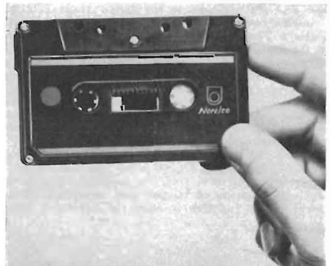
The Philips cassette shown here has a numbered scale over the window to aid in finding a given spot on tape being played.
