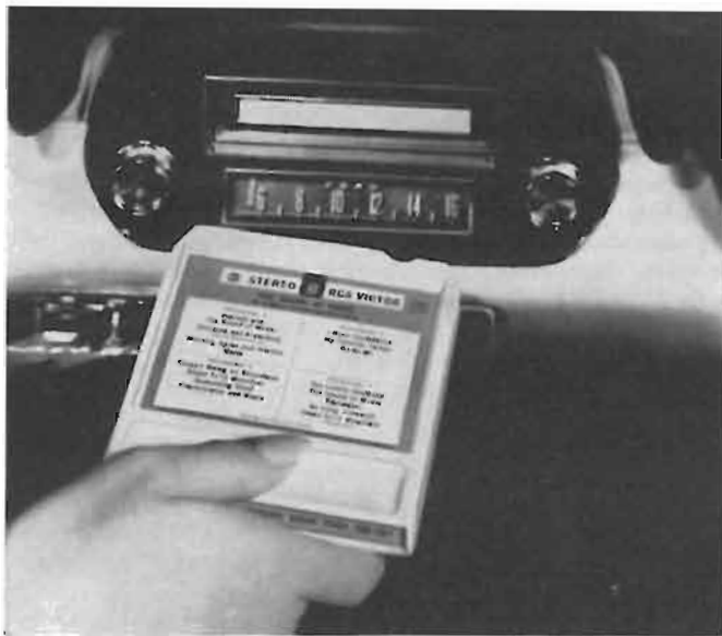
Lear cartridge is about to be inserted into opening above dial of this combination automobile radio and tape playback unit.
