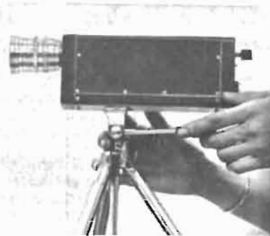
TINY TV CAMERA for space and military use is one of the miracles of integrated circuitry. This one weighs 27 ounces, uses a one-inch vidicon camera tube, and requires only four watts of power.
