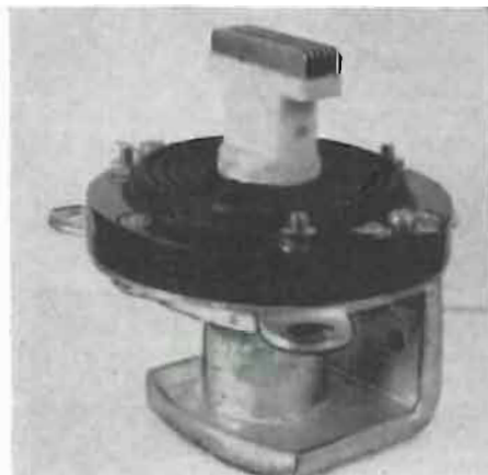
Fig. 4. The wobbulator assembly is a loud-speaker-like arrangement in which a set of capacitor plates are attached to diaphragm. When a 60-Hz low current is applied to voice coil, diaphragm vibrates at this rate and, in turn, moves plates.
